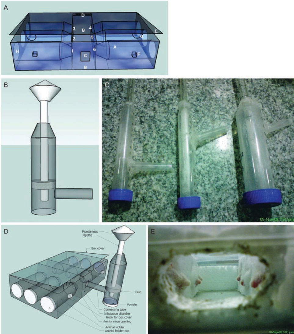
Figure 1. (A) The schematic diagram of the fabricated dosing chamber. A. Centrifuge tubes, B. Dosing chamber, C. Entry port of nebulizer in the dosing chamber, D. Exit port of the aerosol, E. Box cover, F. Hook in the box body, G. Hook in the box cover for tight attachment with the box, H. Wide end of centrifuge tube for placing the animal inside the tube. 1–6: Inhalation ports. (B) Schematic Diagram of fluidization chamber. (C) Comparative illustration of three fluidization chambers. (D) Schematic diagram showing attachment of fluidization chamber with the dosing chamber (inhalation chamber). (E) View of the dosing chamber from the entry port of nebulizer. The noses of mice opened in the dosing chamber are visible in the figure.
